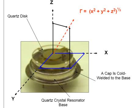
Figure 3. G-forces on a crystal resonator
