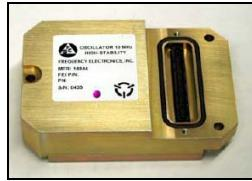
Figure 5. Hard mounted stand-alone g-compensated multiple-output frequency generator unit (Size L x W x H inches 3.7 x 2.5 x 1)
