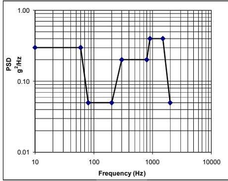
Figure 14. Track vehicle vibration profile
