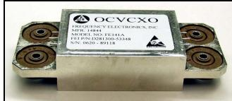
Figure 6. "Soft" mounted stand-alone g-compensate oscillator (Size L x W x H inches 4 x 1.6 x 0.8)
