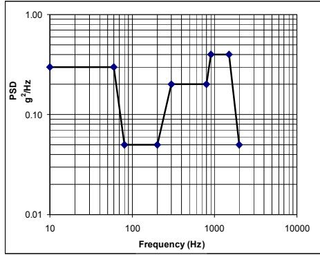
Figure 14. Track vehicle vibration profile
