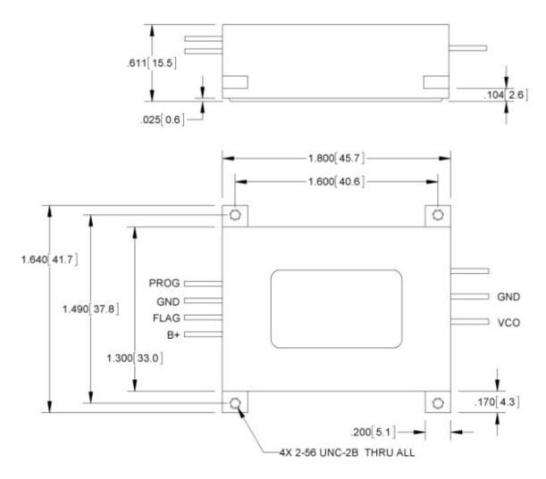
PINOUT: B+ = +12V IN, GND = 12V RETURN, FLAG = HEATER MON., CONTROL (NEG. SLOPE 0-5V) PROG FACTORY, VCO = 0 TO 5V ( $F_0 \approx 2.5V$ ), GND = VCO & RF RTN., RF = 10MHz SINE WAVE OUTPUT
